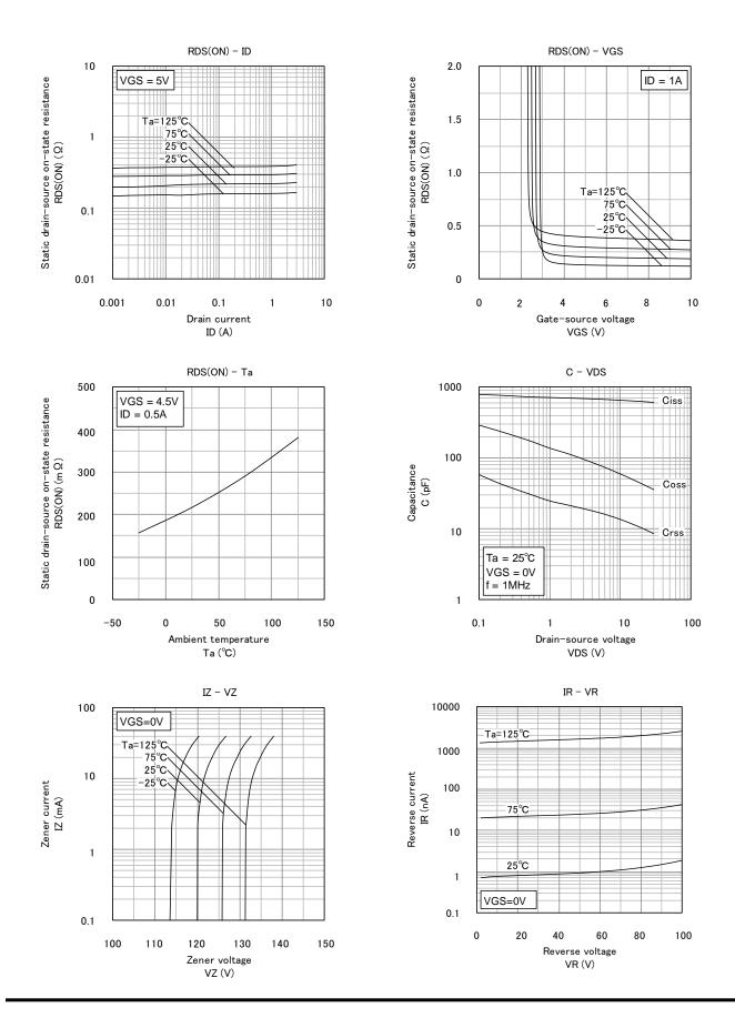
High Speed Switching Silicon N-channel MOSFET
