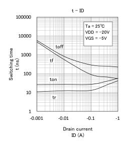
High Speed Switching Silicon P-channel MOSFET
