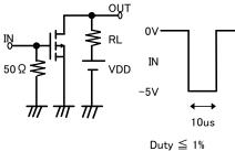
Duty  $\ge$  1% 入力: tr, tf < 10ns VDD=-20V,VG=-5V Common source Ta = 25°C
